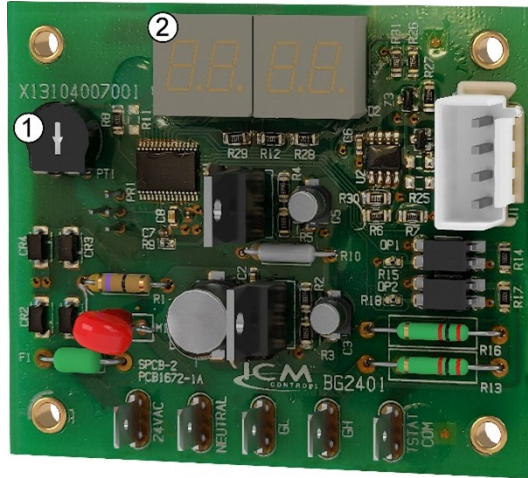
Figure 13. ECM control board
