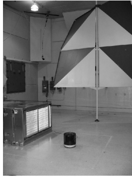
Figure 11. Trane acousticians collect and text sound data
