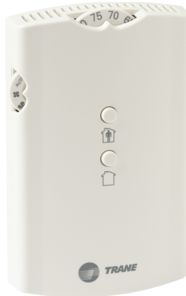
Figure 15. Wall-mounted zone sensor with setpoint dial, OALMH, occupied/unoccupied, COMM (Digit 38 = C)
