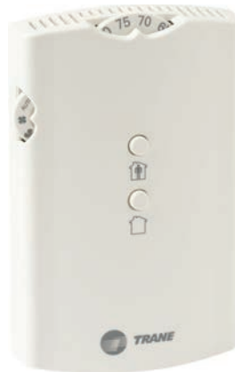
Figure 14. Wall-mounted zone sensor with setpoint dial, OALMH, occupied/unoccupied, COMM (Digit 38 = C)
