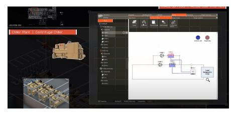
For over 50 years, Trane has developed the TRACE family to provide best-inclass simulation, including component sizing and energy/economic simulation. TRACE can be used to size individual coils to determine air handler or rooftop unit sizing, VAV box sizing, reheat coil sizing, and fan sizing. Then, the software can be used to simulate the as-designed building over a prescribed period to determine energy consumption and cost of operation.
