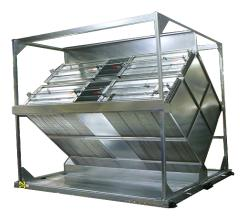
Fixed plate heat exchangers use a series of plates with internal separators to create independent, separate airflow channels. There are a variety of materials used, but aluminum is the most common. The plates and separators are stacked with sealed alternate edges to prevent cross leakage. These exchangers can be made to withstand large pressure differentials. Fixed plate heat exchangers can be designed to handle higher temperatures and have an optional corrosion protection coating.
