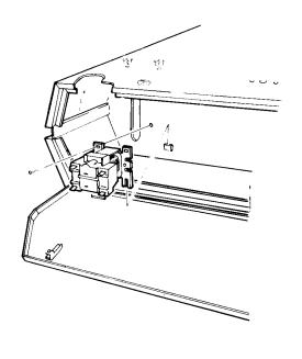
Figure 3 Relay Location on 25KW thru 50KW Units
