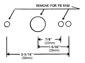
Figure 2 Fan Switch Location on 3.3KW thru 5KW Units
