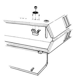
Figure 4 Fan Switch Location on 25KW thru 50KW Units
