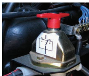
Battery Power Switch
