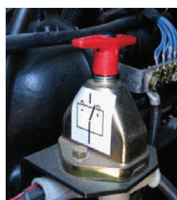
Battery Power Switch
