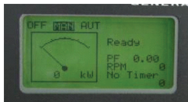
Startup Screen: Press the ► button to select "OFF", "MAN", or "AUTO"
