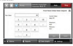
13.To turn machine off, select the STOP button on the 7-inch touch screen. Once the machine has fully stopped, switch disconnect to the OFF position.
