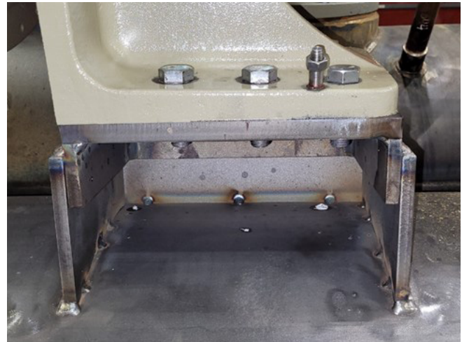
Figure 21. Rear and side plate tacks
