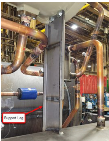
Figure 29. Compressor support leg
