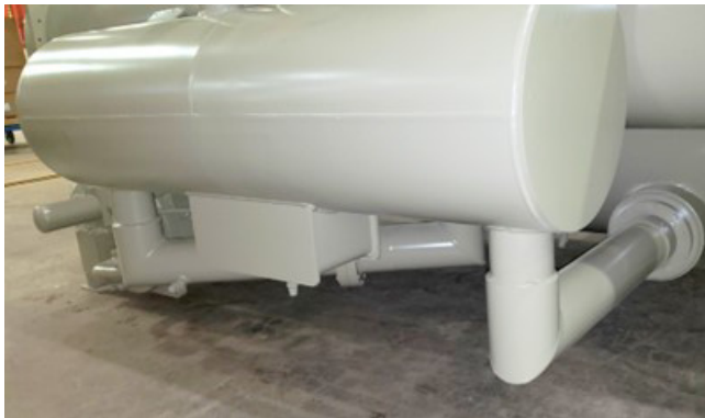
Figure 10. Economizer and liquid line flange
