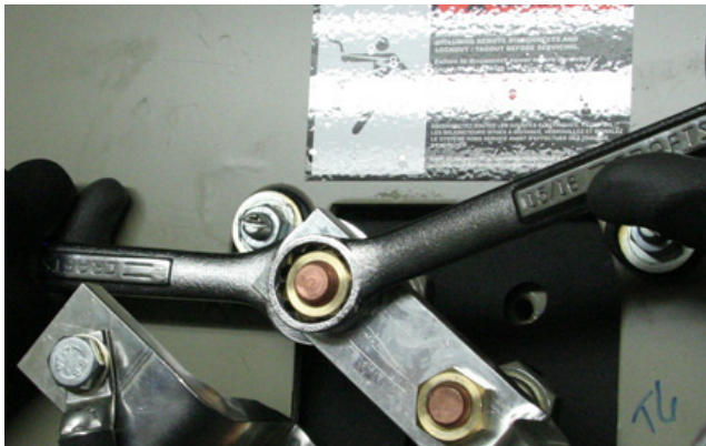
Figure 33. Use backup wrench when removing wire or buss bars from motor terminals
