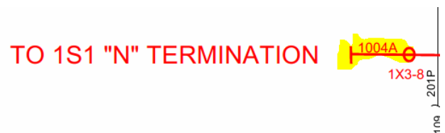
Figure 17. Running new wire from vacant terminal
