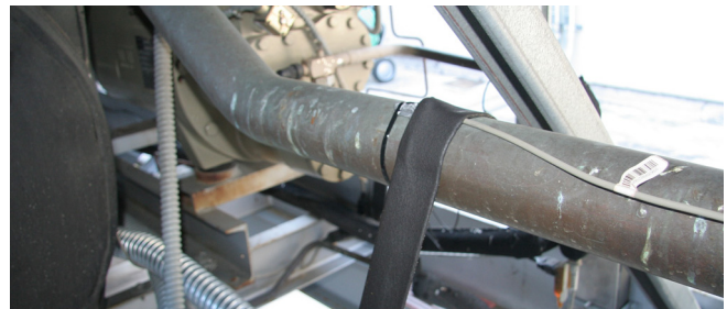
Figure 72. Sensor covered with insulating tape
