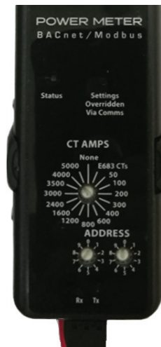
Figure 10. CT AMPS rotary switch and address rotary switch of energy meter
