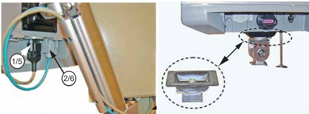
Figure 11. Remove existing display and install new display
