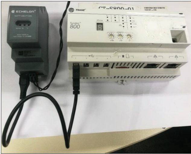
Figure 20. LON wiring, ref. 50712734
