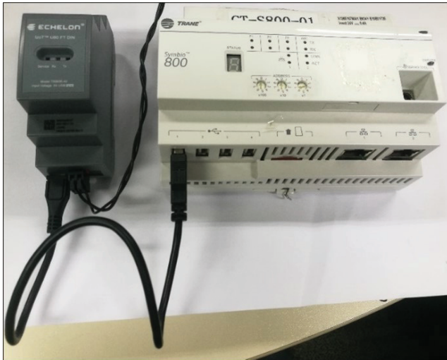
Figure 20. LON wiring, ref. 50712733
