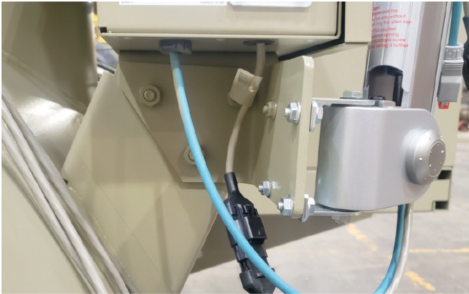
Figure 8. Bolting display arm to the panel
