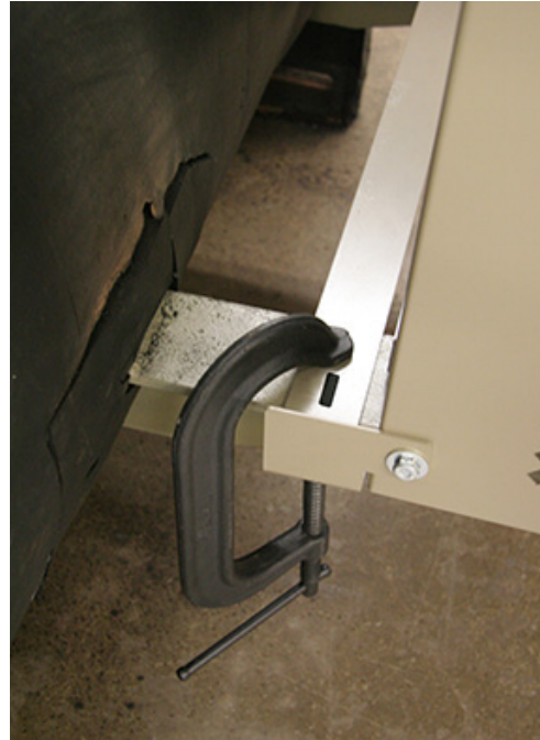
Figure 22. Attaching C-clamp to the adapter bracket
