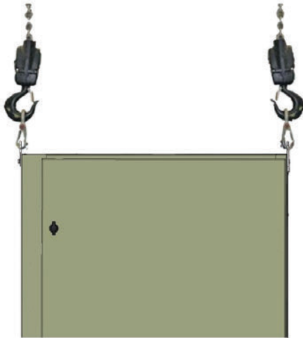
Figure 5. Preferred lifting method using two identical individual hoists
