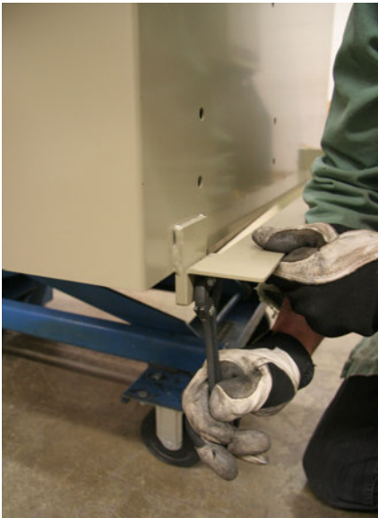
Figure 18. Attaching the other end of the adapter bracket
