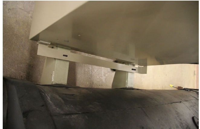
Figure 19. Slots in adapter bracket, for use if the AFDH needs to be moved to avoid interference
