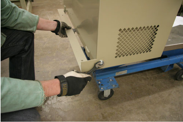
Figure 17. Attaching the adapter bracket to the bottom of the AFDH panel
