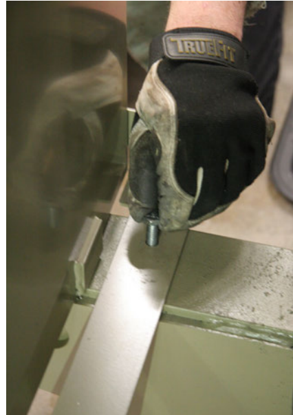
Figure 24. Attaching C-clamp to the adapter bracket
