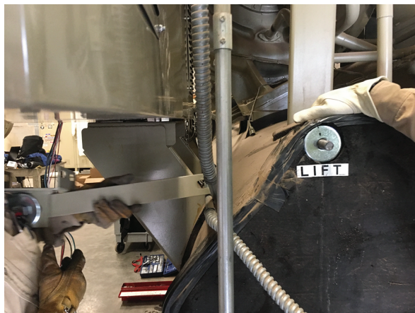
Figure 40. Install linkage subassembly
