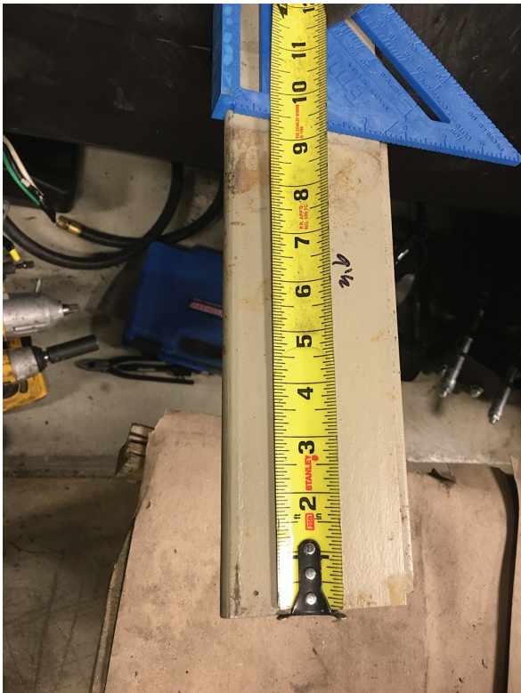
Figure 28. Starter panel brackets markings to trim extra length
