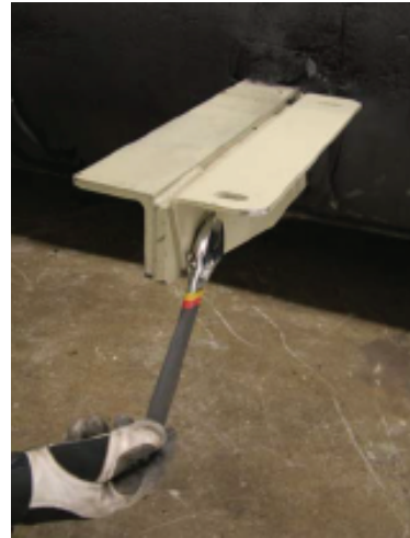
Figure 21. Removing bottom panel bracket from starter panel brackets
