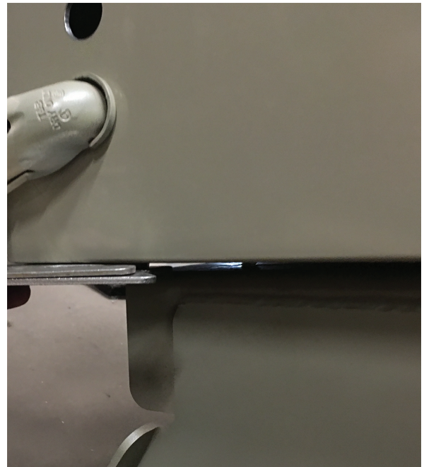
Figure 36. Align the shims
