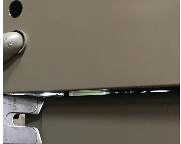
Figure 36. Align the shims
