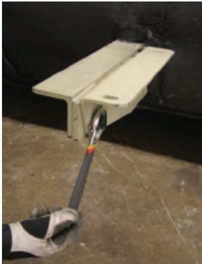
Figure 19. Removing bottom panel bracket from starter panel brackets
