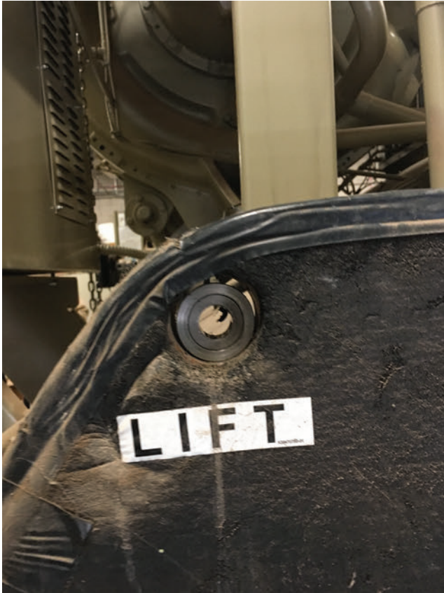
Figure 32. Install linkage subassembly into tube sheet
