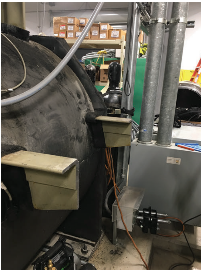
Figure 28. Starter panel brackets after trimming
