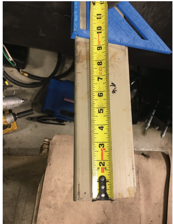
Figure 26. Starter panel brackets markings to trim extra length
