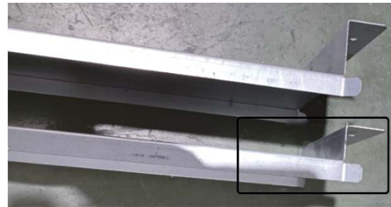
Figure 5. Support plates (shorter used with 7.5 ton)
