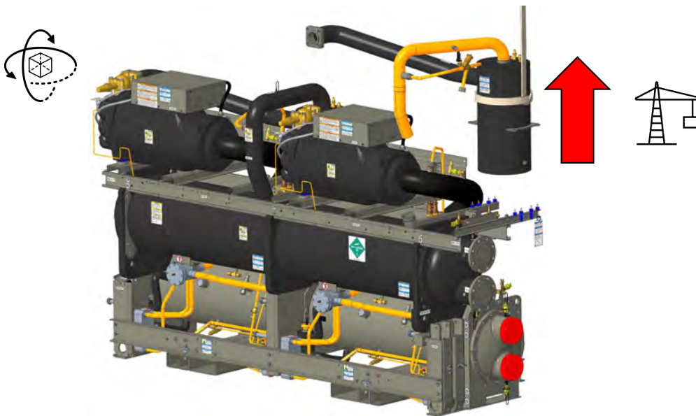
Figure 33. Remove oil separator assembly
