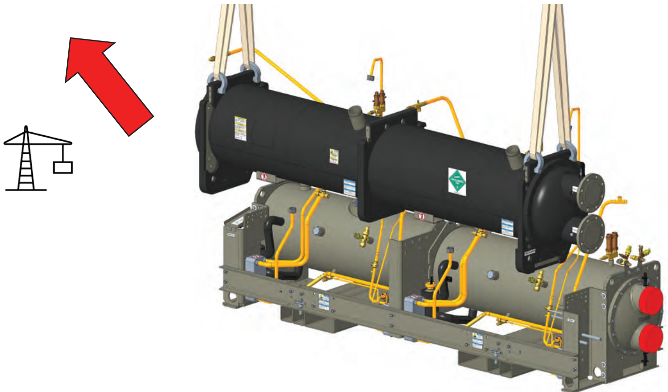
Figure 58. Remove condenser assembly
