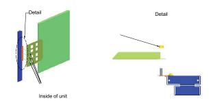
Remove screws from door hinge and door catch. If required, remove screws from standoff brackets.
