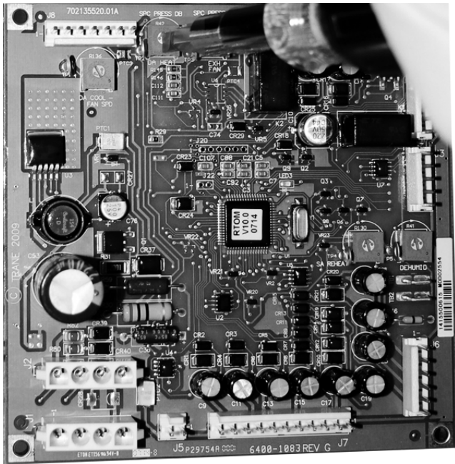
Figure 3. Example of changing potentiometer value on the RTOM
