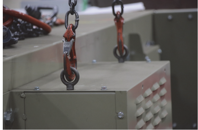
Figure 6. Preferred lifting method using two identical individual hoists
