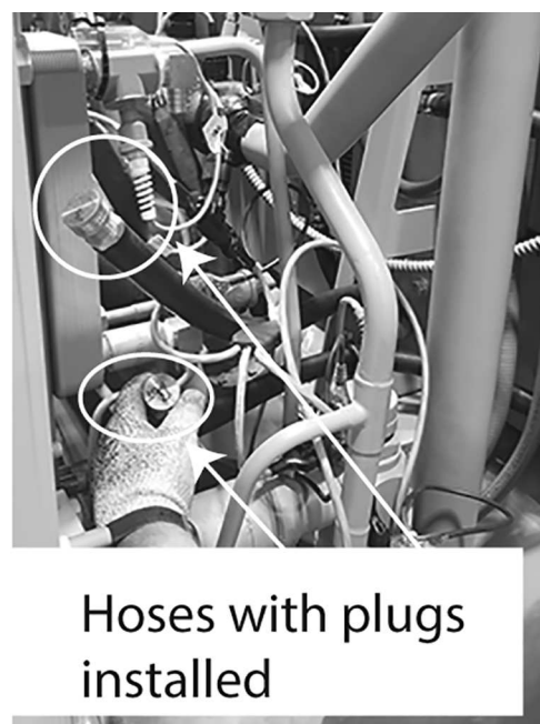
Figure 21. Plugging cooling lines
