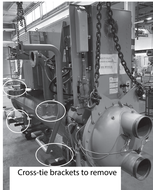
Figure 26. Removing cross-tie brackets
