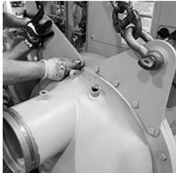
Figure 16. Repositioning lifting bracket
