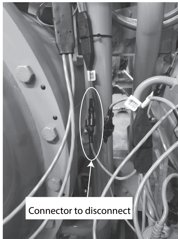
Figure 12. Global connector disconnect
