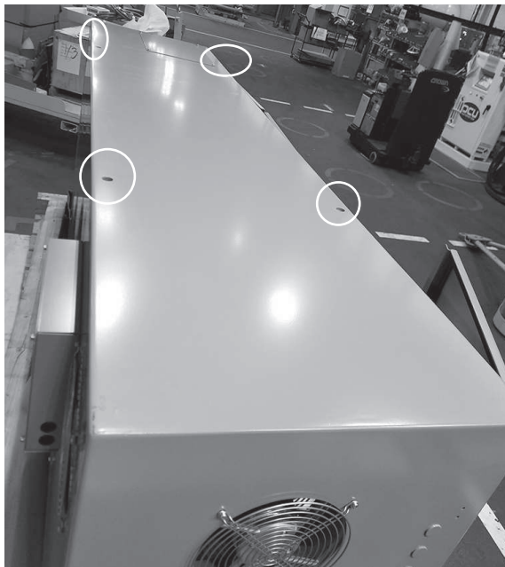
Figure 41. Lifting locations for the control panel
