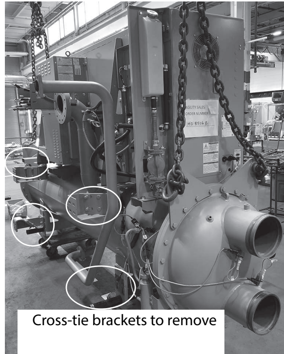
Figure 26. Removing cross-tie brackets
