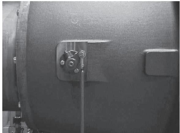
**Figure 11. Vane actuator level on interstage**
