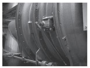
Figure 12. Vane actuator operator mechanism
