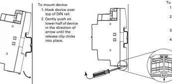
To remove/reposition device 1. Disconnect all connectors before removing or repositioning. 2. Insert screwdriver into slotted release clip and gently pry upward with the screwdriver to disengage the clip. 3. While holding tension on the clip, lift device upward to remove or reposition 4. If repositioned, push on the device until the release clip clicks back into place to secure the device on the DIN rai
