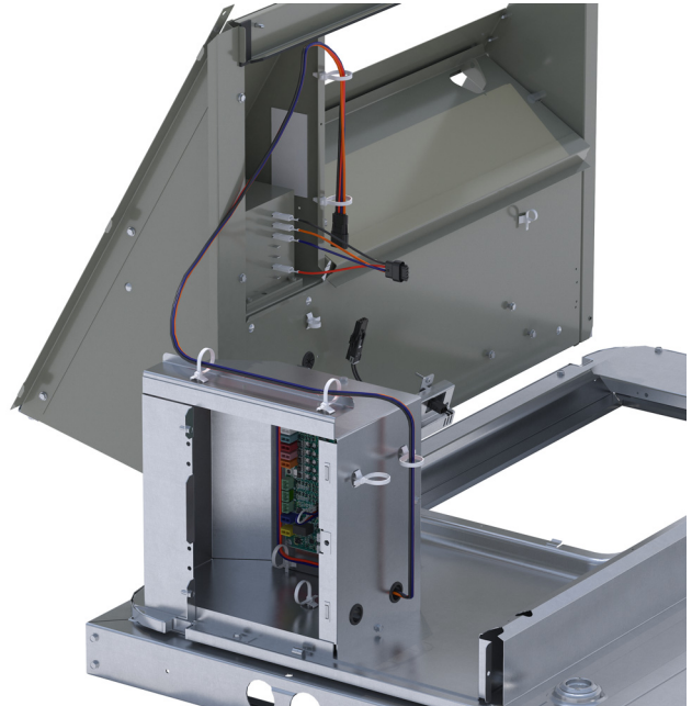
Figure 11. Wire routing to fresh air options module
