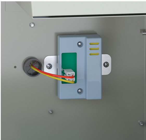
Figure 1. Route red and yellow wire to humidity sensor
