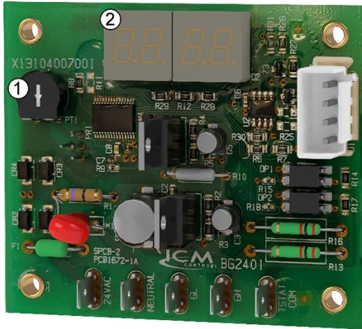
Figure 26. ECM control board
