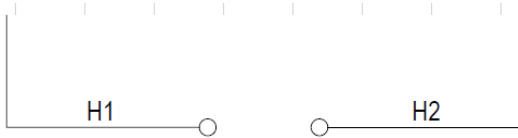
Figure 61. Deluxe controls humidistat connections between wires H1 and H2 in control box low voltage connection (0.5 to 5 ton)
