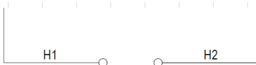
Figure 31. Deluxe controls humidistat connections between wires H1 and H2 in control box
