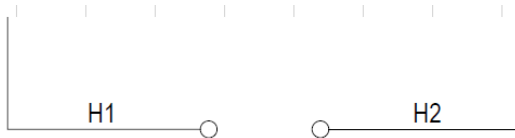
Figure 62. Deluxe controls humidistat connections between wires H1 and H2 in control box low voltage connection (0.5 to 5 ton)
