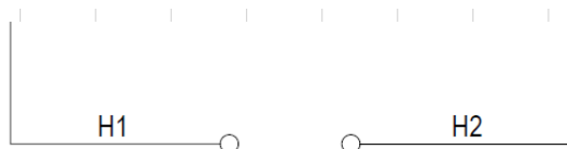
Figure 62. Deluxe controls humidistat connections between wires H1 and H2 in control box low voltage connection (0.5 to 5 ton)
