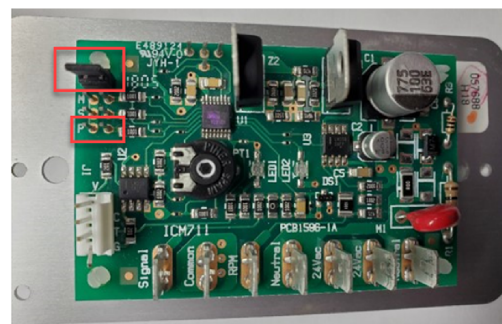
Figure 30. ECM control board 2-10 Vdc input signal shunt placement
