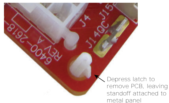
Figure 66. Remove PCB
