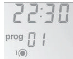
Figure 52. Setting the switching ON time
