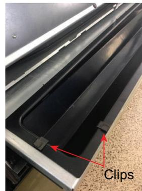
3. Remove drain pan for cleaning.
