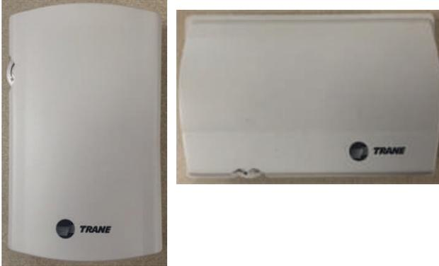
The fan speed control can be used to provide simultaneous fan speed customer requests in addition to external controller fan speed request. The wall-mounted option is low-voltage and has three 24-volt relays using a factory-wired transformer and relays to control the fan motor.
