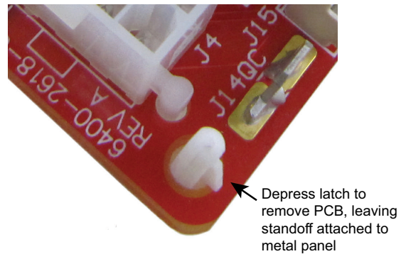
Figure 77. Remove PCB
