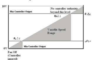
Figure 73. Example 2:  $\Box F \bot r$  set too high but  $A \Box S c$  set correctly
