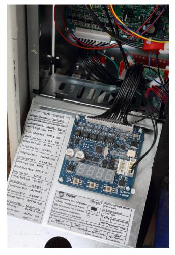
The motor control board features a nested menu integrated user interface (UI) that supports:
