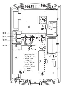
The sensor for a wireless zone sensor (WZS) has four LEDs: LED1, LED2, LED3, and LED5 and a test button. Locations are shown in the following figure.
