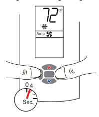
Note: If you try to access a feature that is locked, the locked symbol will appear on the display. If you press a keypad button to try change a locked setting, the locked symbol will flash.
