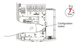
The display will change to configuration mode. When the sensor is in configuration mode, a wrench symbol appears on the display and the menus are separated by lines, as shown in Figure 52, p. 44.
