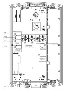
The sensor for a wireless display sensor (WDS) has test symbols and error codes that appear on the display, and a test button. Locations are shown in the following figure.
