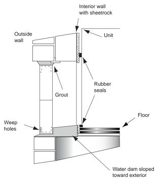
Grout the top and bottom of the wall box frame as noted. A sloped water dam located in the space between the unit and wall facilitates moisture drainage. Grouting at the ends of the intake box will complete the seal between the wall box frame and the masonry opening.
