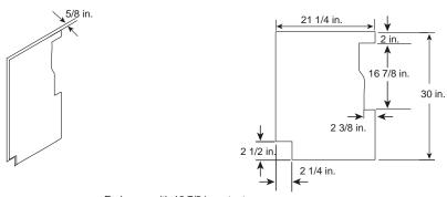
End cover with 16 7/8 in. cutouts for 4-pipe, dynamic air, and wall fin applications
