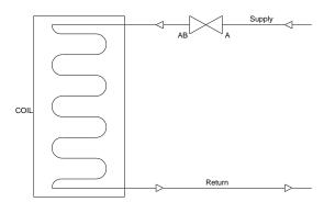
**Note:** The actuator must be mounted between 0 and 45 degrees from horizontal. Do not install with actuator below pipe.
