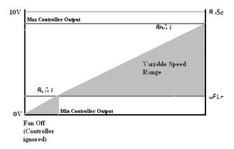
Figure 74. Example 3:  $\Box F \Box r$  set correctly and  $R \Box S c$  set correctly
