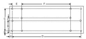
There are 1/2-inch mounting or anchoring holes located on the back of the unit on each end.
