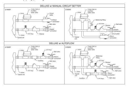
Figure 16. Supply and return connection
