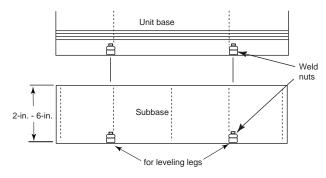
Set the unit on the subbase and fasten with four, 0.375-16
