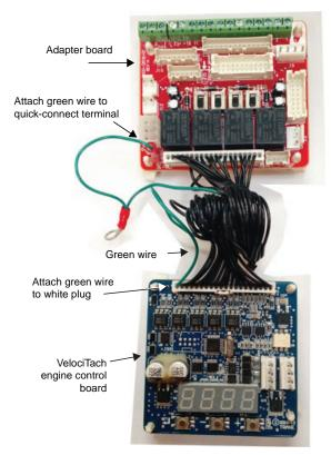
4. Ensure that the new VelociTach™ motor board controller is configured to match the configuration label that is present on the unit. It is necessary to configure the VelociTach™ board to avoid improper operation of the unit, discomfort to the end user, and loud fan operation.
