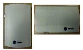
The fan speed control is available for units that do not have Trane factory-mounted control packages. This variable fan speed option is low-voltage and has three 24-volt relays using a factory-wired transformer and relays to control the fan motor.
