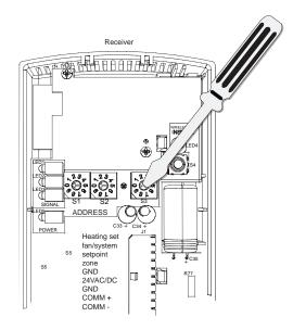
Set the three rotary address switches (locations S1, S2, S3) on the sensor to the same address as the receiver.
