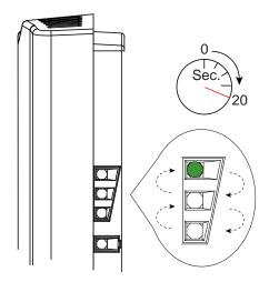
After the channel scan is finished, LED3 begins blinking (oneblink pattern) to show that the receiver is ready to be associated with a sensor.
