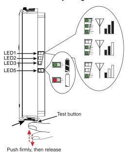
3. For model WDS, determine the signal strength and battery status by viewing the symbols on the sensor display. Record the results in your commissioning statement.
