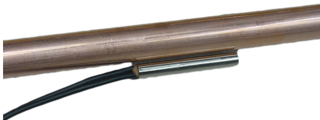
Figure 30. Close-up view of the entering water temperature sensor
