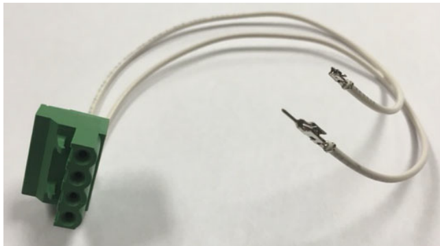
Figure 43. Connecting wires to terminal
