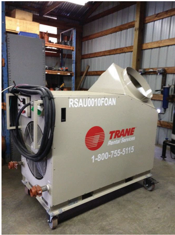
Figure 7. RSAU0010F1 (2 supply style AHU)
