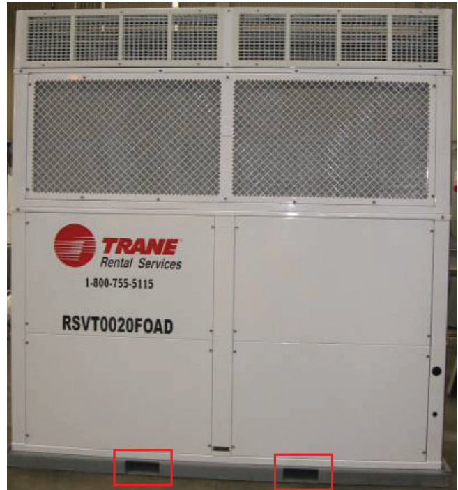
Figure 20. 20 ton vertical air conditioning unit and forklift pockets
