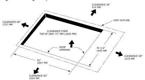
Figure 8. Cooling with optional electric heat — downflow unit clearance
