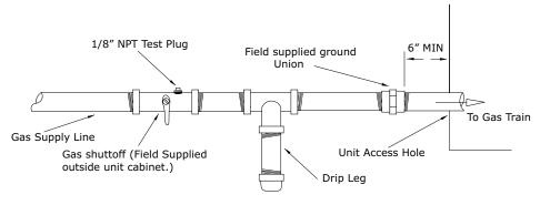
Figure 29. Typical unit gas train configuration
