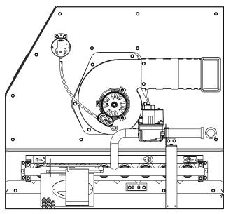
Remove six screws from manifold bracket. See the following figure.
