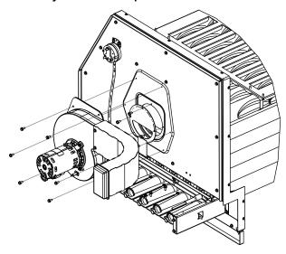
Figure 22. Remove screws from inducer blower assembly
