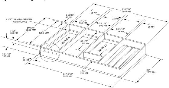
Figure 6. Cooling with optional electrical heat — roof crub
