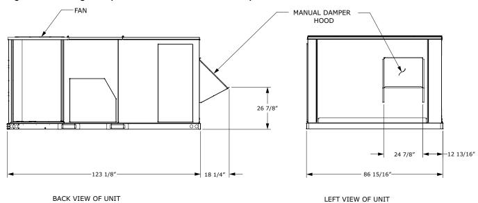
Figure 10. Cooling with optional electric heat — manual damper
