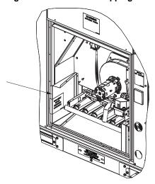
Install the vent hood on the gas heat panel using the screws removed in Step 1. Make sure it is properly secured to the panel.
