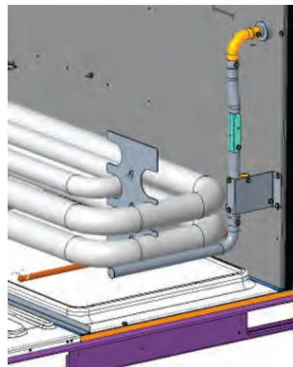
Figure 67. DAS tubing after conversion to horizontal
