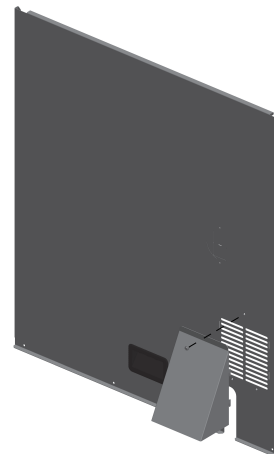
Figure 14. Vent hood installation
